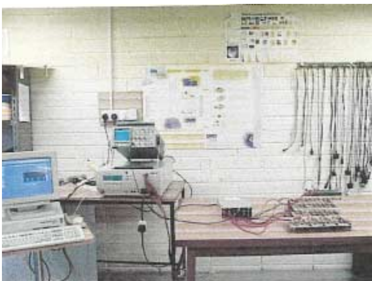
Figure A4. EFT / Surge immunity test set-up
